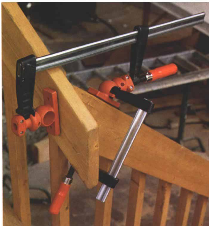
Irregular angle clamp. Made by Bessey, this two-jawed clamp brings together parts that meet at odd angles, such as this stair railing. Photo by Felix Marti.
