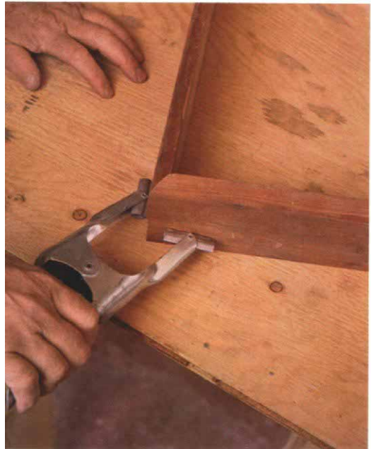
Spring clamp at the corners. A pivoting-jaw spring clamp has tiny teeth that secure mitered corners, 90° or otherwise.
