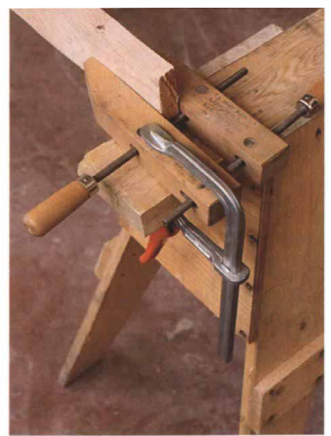
Clamp-on sawhorse vises. A sturdy anchor at one end of the sawhorse can make it a lot easier to plane the edge of a board. Stanley's steel vise (photo below) has prebored holes for attaching wooden jaw liners. Bessey's version has plastic jaws that ride on a pair of guide bars (bottom photo). The bars can be removed, allowing the jaws to swivel and thereby accommodate irregular shapes. A handscrew clamped to the end of a sawhorse can also make a serviceable vise (photo above).
