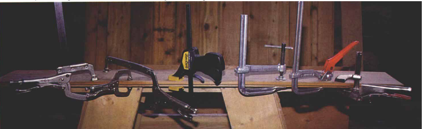
Beyond the C-clamp. Locking clamps, pistol-grip bar clamps and quick-action lever clamps exert similar loads as C-clamps do but do it faster and one-handedly. Left to right: American Tool Co.'s bar clamp has a sliding
