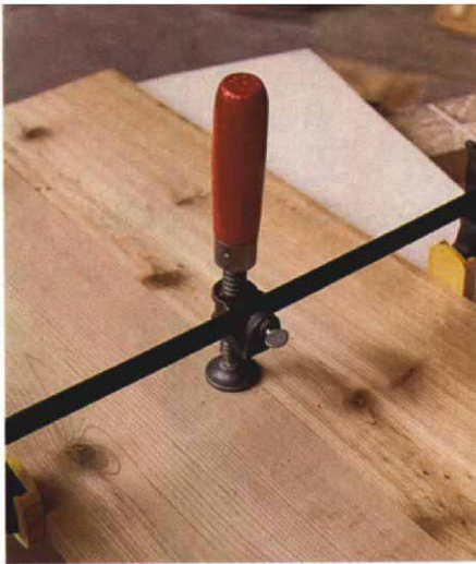
Edge clamp in the field. Affixed to a bar clamp, an edge clamp can exert downward pressure to counteract the tendency of edge-glued boards to bow upward.
