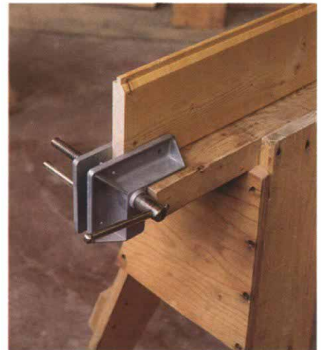
Clamp-on sawhorse vises. A sturdy anchor at one end of the sawhorse can make it a lot easier to plane the edge of a board. Stanley's steel vise (photo below) has prebored holes for attaching wooden jaw liners. Bessey's version has plastic jaws that ride on a pair of guide bars (bottom photo). The bars can be removed, allowing the jaws to swivel and thereby accommodate irregular shapes. A handscrew clamped to the end of a sawhorse can also make a serviceable vise (photo above).
