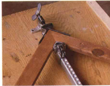
Cylindrical jaws. Hafele's top-spanner bar clamp (below) has PVC-wrapped cylindrical jaws that can get a bite on workpieces that come together at any angle between 45° and 135°. Photo courtesy Hafele.
