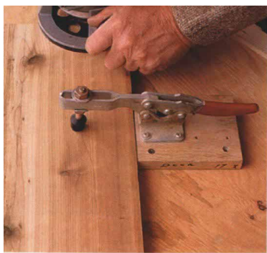
Hold-down. De-Sta-Co clamps apply a point load by way of a lever-activated cam.
